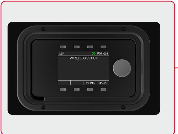
**PRIMARY/CLONE** When selected, ALLEGRA-C™ will become the primary fixture and a network symbol will be displayed on the info bar. In this mode, any ALLEGRA-C™ connected to the primary, via the DMX sockets, will copy its behaviour.
