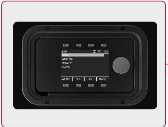
**WIRELESS** In wireless mode, ALLEGRA-C™ will attempt to pair with a CRMX wireless transmitter and the wireless symbol on the info bar will flash. Once paired, the wireless symbol will become solid green. To un-pair, press the unlink button and ALLEGRA-C™ will immediately start to search for a new transmitter. Do not use wireless mode with wired DMX connected, or the fixture may behave erratically.
