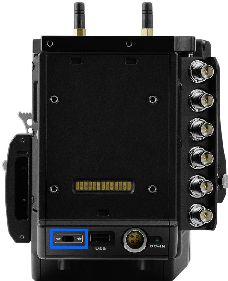
*Figure: Auto Boot on Power Switch*
