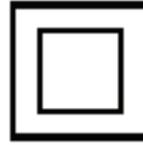
Products marked with this symbol are class 2 devices. These devices are not provided with a grounding type plug.
